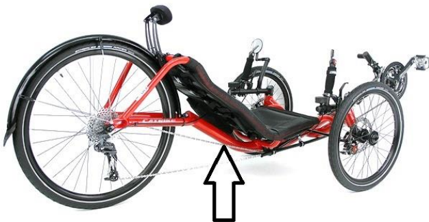
On space frame models Expedition, 700, Pocket S/Ns are on the bottom side of the main frame.
