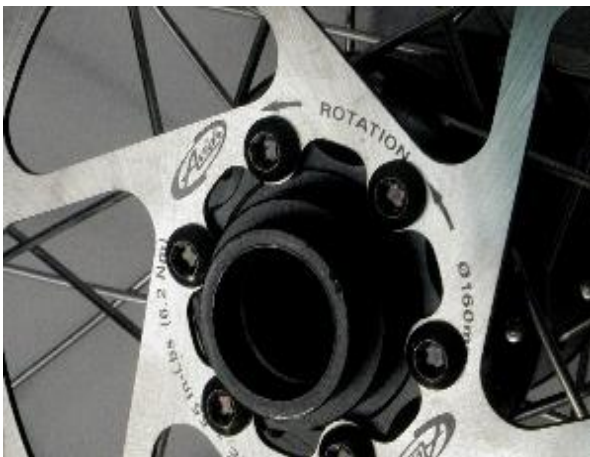
Direction of rotation shown on brake rotors
