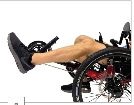
When the rider places the ball of the foot on the pedal or clips their shoe in, they should have a slight bend in the knee. Make sure boom clamp quick releases are tightened properly and all seat straps are tight and restrained before riding.
