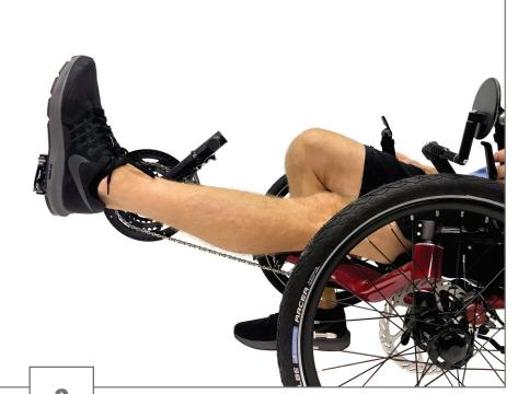
Adjust the quick release boom until the rider's heel sits on the pedal with their leg fully extended. Make sure the rider does not have to reach for the pedal. Booms can be cut to accommodate shorter riders, always leave 5 inches of the boom inside of the frame.
