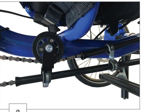
Proper chain routing and chain tube position on Villager. Note the P-clamp and chain tube on the chain keeper.
