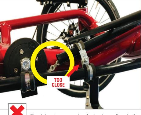
The tube clamps are too far back resulting in the chain rubbing the bottom of the upper chain tube.
