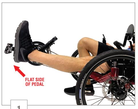
Have the rider sit in their normal riding position and align one of the crank arms with the boom. Have the rider extend their leg and place their heel on the flat side of the pedal that is extended the farthest from the end of the boom.
