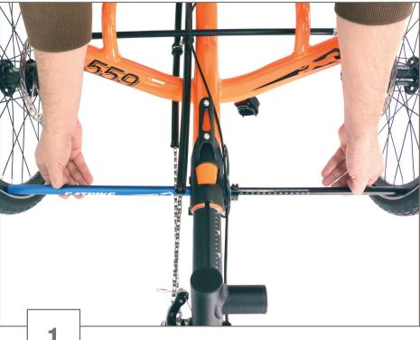
Measure the front of the wheels first (from the rim for better accuracy), at axle height, then measure the back.
