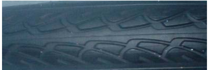
On the tire, the "arrows" point left, giving you direction of rotation.
