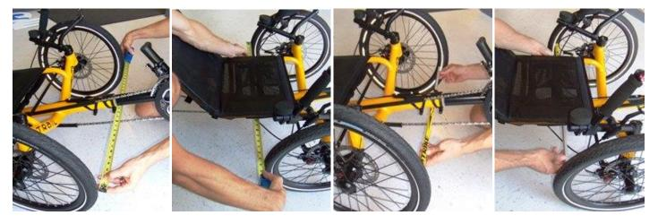
It's very important to get this right...if you have a quarter inch of toe your tires will wear out very quickly and handling performance will be degraded. Proper toe-in will also affect rolling efficiency. Too much toe-in (greater than 1/16" or toe-out where the front of wheel is wider than the rear) are to be avoided as either incorrect setting will significantly reduce rolling efficiency.
