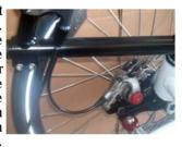
Thread the end of the cable through the fittings in the brake actuating arm. The ferrule fits under the rubber boot. Loosen the cable clamp bolt, put the cable under the clamp plate, pull it taut and retighten the bolt. Using a bicycle cable cutter (preferred) or a SHARP pair of wire cutters cut the brake cable so that a few inches extend beyond the clamp bolt.
