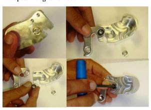
Insert the quick release into the rear wheel, put the wheel into the dropouts, tighten and close the quick release.
