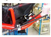
Note the chain routing above there are two chain guide tubes with the top tube running above the cross member (drive) and bottom guide tube (return) running beneath the cross member. The drive part of chain runs underneath the black guide pulley and over the top of the chain ring.
