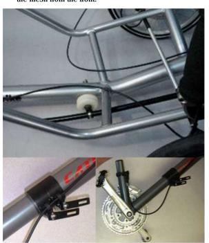
• Installation of the cables at the derailleurs is similar to the installation on the brakes. Put a ferrule on the end of each cable housing. Thread the cables into the derailleurs, pull them taut, clamp them down, trim and seal the ends. Before you clamp the rear derailleur cable in place, screw the barrel adjuster on the derailleur in as far as it will go, then back it off 1 to 1-1/2 full turns. Note that there is no adjuster on the front derailleur.
