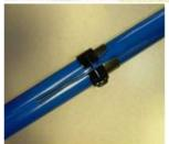
When you install the boom, make sure the plastic sleeve is properly placed, flush with the end of the frame under the collar. Once the boom is in place, tighten the quick release only enough to keep it from sliding: you'll be adjusting it later.
