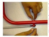
Thread each tie rod end in half way before mounting it. This will give you the most "travel" when adjusting toe later. Attach the rod end bearings to the handle bars. Next, attach the rod end bearings to each spindle.
